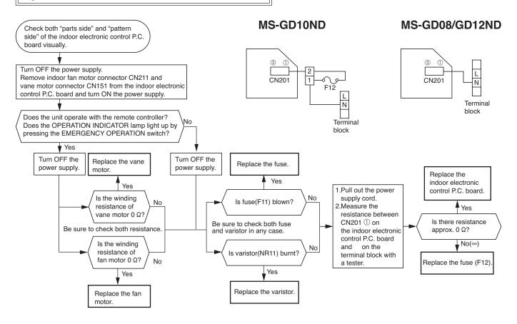
When both OPERATION INDICATOR lamps flash ON and OFF every 0.5-second. Indoor unit and outdoor unit don't operate.
